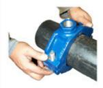
Fit the bottom half of the Pipe Tee and assemble the bolts. Make sure that the square shoulder of the bolt engages in the slot in the bolt pad. Fit the nuts and washers to each bolt and finger tighten both nuts to leave equal gaps between the top and bottom half bolt pads.
