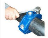
Tighten both joint bolts in turn ensuring equal joint gaps to a torque of 150 Nm which is sufficient to seat the gasket against the pipe. Increased bolt torque will not improve sealing and may cause distortion or failure.
